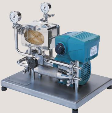
The Alfa Laval LabUnit M10 comprises one Alfa Laval LabStak™ module as well as cross-flow pump, heat exchanger, valve and pressure gauges.
