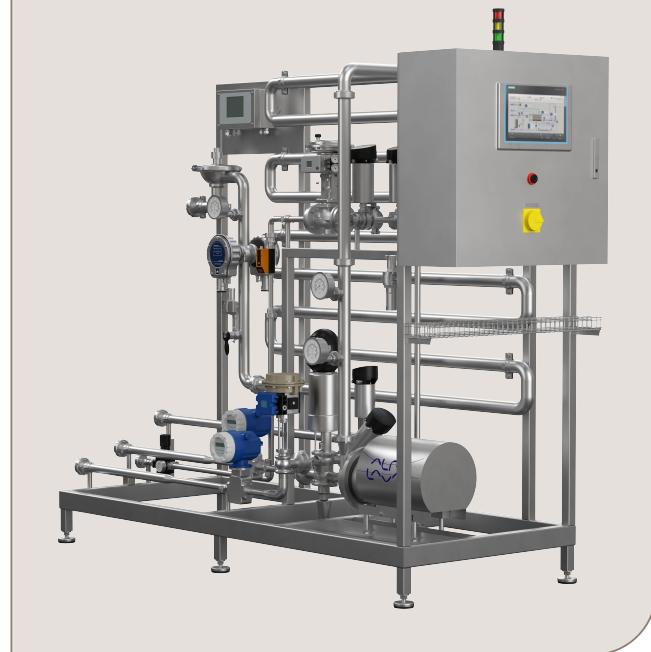
A control valve regulates the CO<sub>2</sub> flow to keep a constant CO<sub>2</sub> content in the product. A PLC controls the plant operation.
