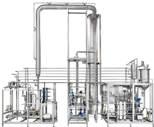
The process sections of Alfa Laval De-alcoholization Module – degassing and aroma recovery (right), alcohol removal & culinary steam generation (middle) and condensate cooling (left).
