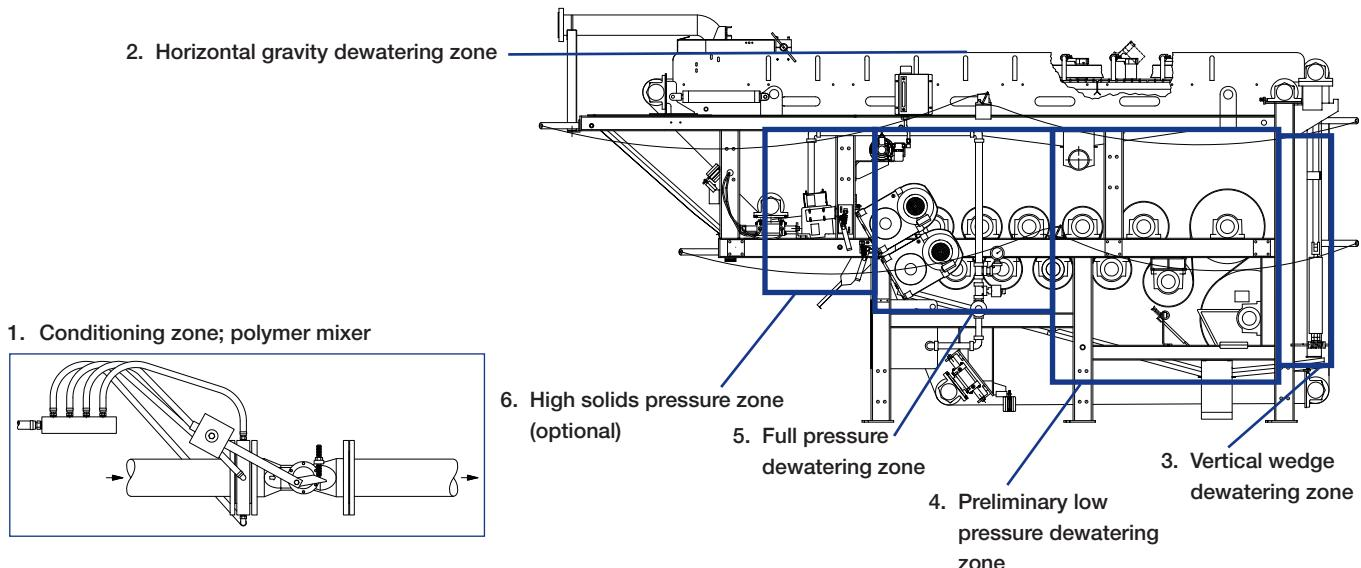
**1. Conditioning zone** – optimized dewatering begins with the proper conditioning of the slurry. Each unit is equipped with a proprietary variable orifice in-line polymer mixer that combines polymer and slurry instantly to facilitate rapid flocculation. This design allows the unit to use the lowest dosage of polymer while achieving the highest cake solids.
