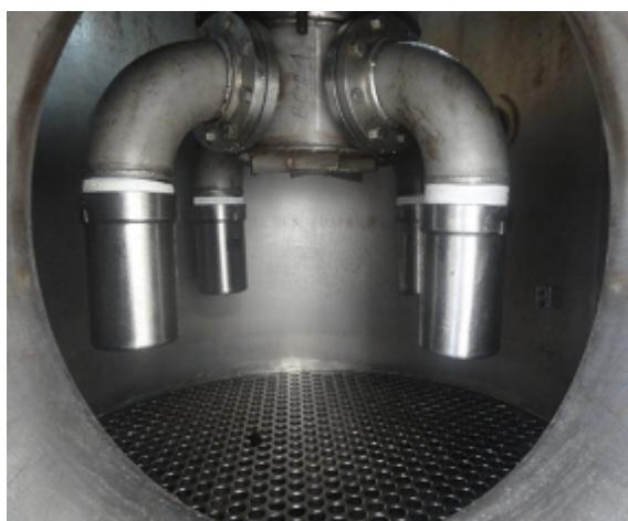
distributor available in Alfa Laval FilmVap evaporators is the jet distributor, fitted with solid cone spray nozzles. The size and quantity of these nozzles
